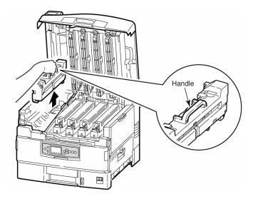
5. Unpack the new fuser and lower it into the printer.
